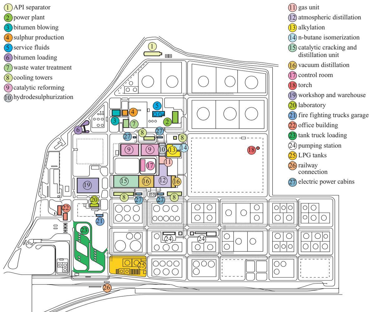
Fig. 11. Typical ground plan of a refinery of the second half of the Twentieth century.
